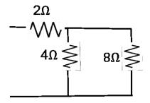
Step 4: combine  $4\Omega$  and  $8\Omega$  resistors [parallel]:  $(1/4\,\Omega+1/8\,\Omega)^{-1}=8\,\Omega/3$
